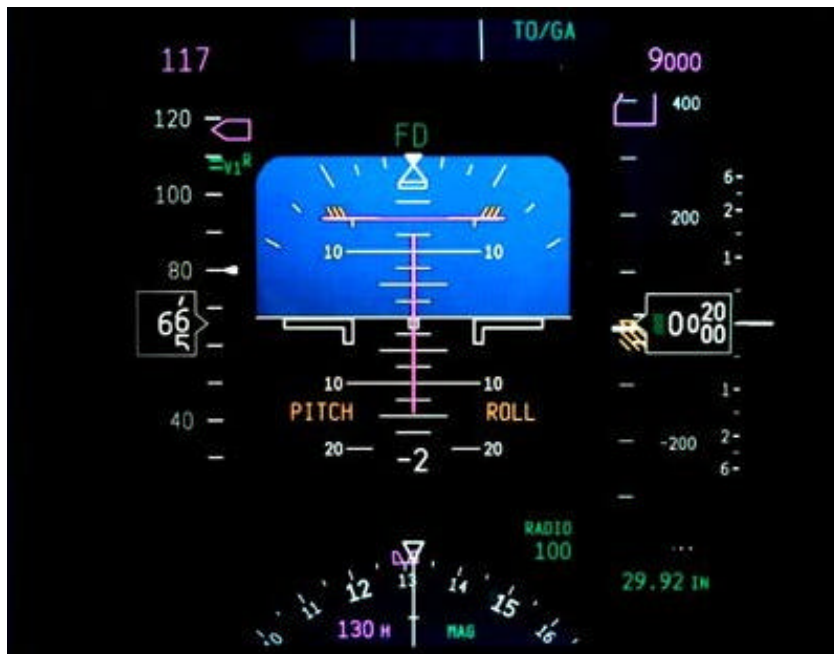
Figure 9. A primary flight display. The airspeed tape is on the left, altitude tape on the right.
