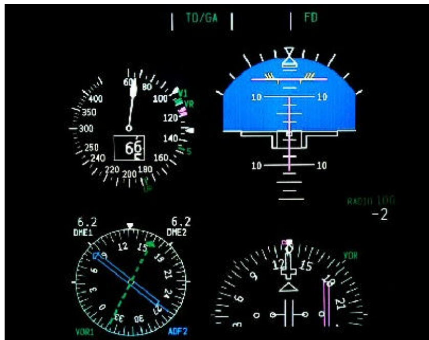
Figure 10. The primary flight instruments in the Boeing Next-Generation cockpit. The digital recreation of the electromechanical mach/airspeed indicator (MASI) is at the upper left.
